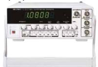
The Voltcraft FG 8210 function generator outputs signals from 0.1Hz up to 10MHz with different signal forms and adjustable amplitude and symmetry. The following waveforms are available sine, rectangle, triangle with DC to TTL-synchronous output, a linear wobble function, DC offset setting, and voltage-controlled frequency setting (VCF). The generator also has a frequency counter up to 100MHz.
