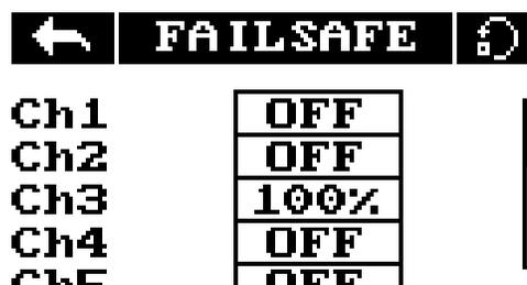
You can set the failsafe position for all channels with the **[All channels] button at once. To do so:**
