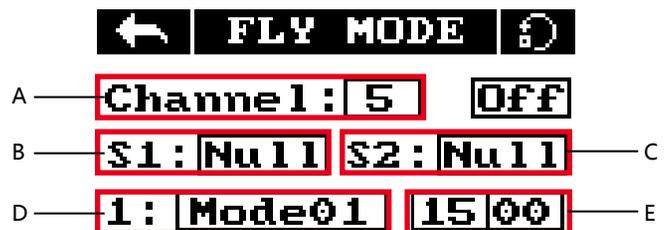
Different fly modes are assigned using combinations of switches. A 2-way switch will enable you to switch between modes 1 and 2, two 2-way switches will enable you to 4 fly modes, two 3-way switches will allow you to switch between all 9 fly modes. Use the table below to see which positions are assigned to each mode.
