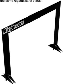
Airgineers Micro Class Gates can be laser cut from 5mm acrylic. Visit **www.airgineers.co.uk** to download the files for laser cutting.
