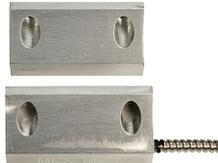
Heavy duty magnetic contact switches in a short, wedge-shape extruded aluminium housing. The switches have a 22in armoured cable and come with a matching wedge-shape magnet. Ideal for use as heavy duty door contacts for industrial and commercial applications in harsh environments.
