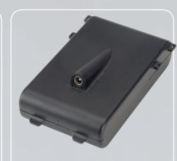
NAO Humanoid Robot Spare Rechargeable Battery and Charger A spare or replacement rechargeable battery pack for the NAO humanoid robot.
