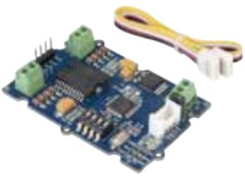
**Grove - I2C Motor Driver Dual Channel 2A Per Channel**
