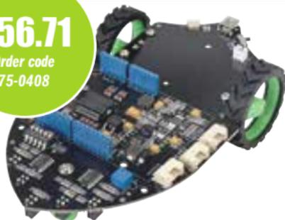
**Shield Bot V1.1 Arduino Compatible with Grove Connectors**
