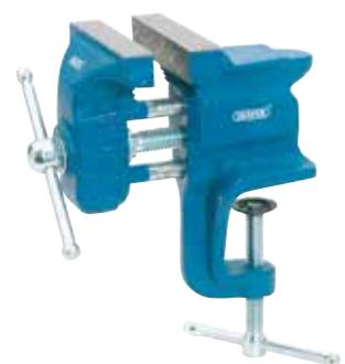
Cast iron with serrated curved jaws. Bench clamping screw 40mm capacity manufactured from zinc plated carbon steel. Display packed. Display carton.
