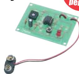
The 555 Astable/Monostable PCB project has been designed specifically to support and integrate with teaching schemes for **Key Stages 3 & 4**. Instruction details are available for free download at [www.rapidonline.com](http://www.rapidonline.com).
