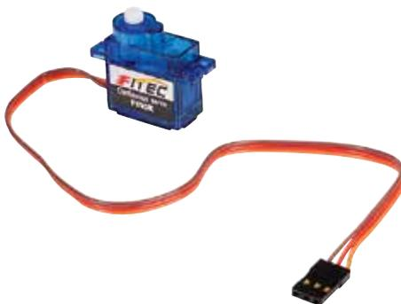
The **FS90R** is an analog micro servo that is capable of continuous rotation clockwise or anti-clockwise, as opposed to moving to a set position. The servo is ideal for the beginning roboticist and is perfect for use with the Motor Shield for **Arduino**. The servo can be controlled using any servo code, hardware or library and to control with an Arduino, just connect the orange control wire to pin 9 or 10 and use the Servo library included with the Arduino IDE.
