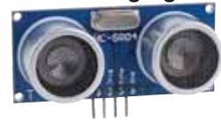
The HC-SR504 is a non-contact ultrasonic ranging module with a 20 to 4000mm range. The module includes ultrasonic transmitter, receiver, and control circuit - all on a compact circuit board.
