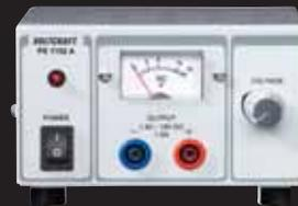
This electronically regulated linear power supply has a fixed current limit at 1.5A. The PS-1152A is protected against overheating and short circuit. The PSU is convection cooled.
