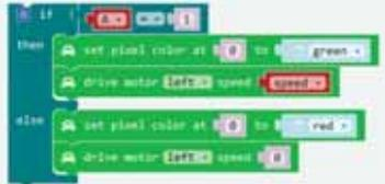
The first **if** statement is checking to see if the variable **A** is equal to 1 (i.e. button **A** is pressed). If **A** = 1 then the pixel at address 0 is set to green. Don't forget, it won't actually change colour until the program gets back to the **show** command.
