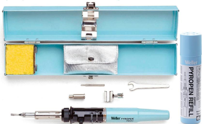
Powered by Butane gas, this Pyropen offers soldering iron, hot air blower and blow torch options. It has a short heat up time and can be refilled in seconds from a refill cylinder. A sight glass shows the level of gas in the reservoir. Temperature control is achieved by increasing and decreasing the gas flow.
