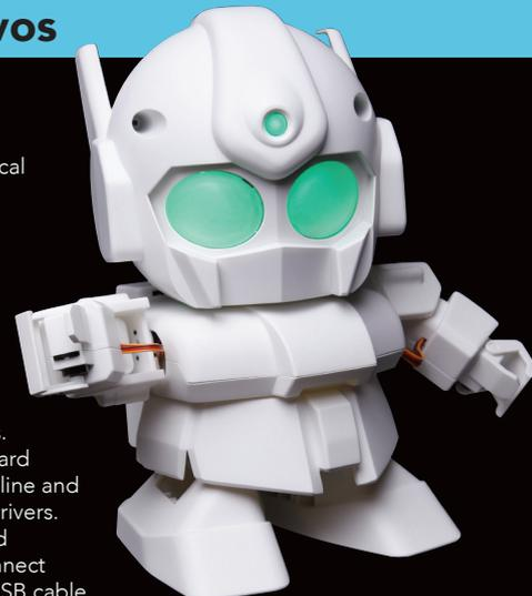
Controlling the robot is very simple using its built in set of pre-programmed motions which include walking, waving, grasping etc. Each motion is accompanied by a dynamic eye colour change. Since the controller board is Arduino UNO compatible you can use the official software as a starting point for your own functions or start again from scratch to control Rapiro your own way.
