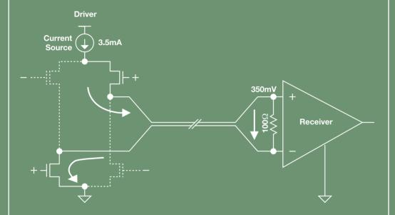
The low common-mode voltage (the average of the voltages on the two wires) of about 1.25V allows LVDS to be used with a wide range of integrated circuits with power supply voltages down to 2.5V or lower. The low differential voltage means that LVDS consumes very little power compared to other systems. For example, the static power dissipation in the LVDS load resistor is 1.2mW, compared to the 90mW dissipated by the load resistor for an RS-422 signal.
