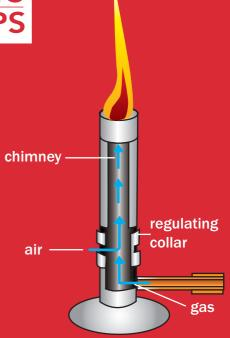
With the regulating collar closing the air holes, the flame is yellow and is relatively cool. With the regulating collar exposing the air holes, the blue flame roars and is at its hottest. The hottest point is just above the inner cone of the flame.
