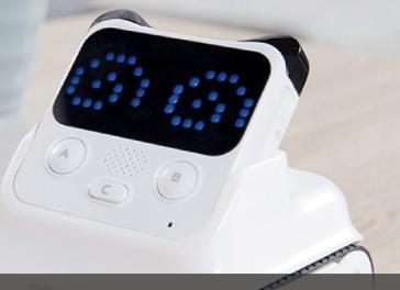
This program helps recognize and classify waste. Based on the recognition result, Codey's LED display will show a sign with the lights in front of one of the waste bins turning on to tell you which bin you should throw your waste in.
