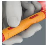
The recesses in the fast-rotating sleeve allow resistance to be generated by finger force. This allows the ratchet mechanism to be used even at low resistance of the screw.
