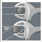
Thanks to the corner-width rectangular prisms in both jaws of the double spanner, a return angle of only 30° can be achieved.
