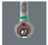
The Joker's holding function means that nuts and bolts can be held in the open end and easily positioned where they are needed. Fastening on to the thread can then be done quickly and safely, thanks to the innovative special stop-plate which holds the fastener. No more time-wasting searches for dropped nuts and bolts! After applying and positioning the nut or bolt, fastening can begin immediately - no additional tools required.
