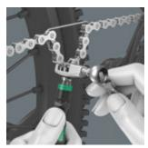
With the included chain tools, chains can be loosened and reconnected; for opening and closing bicycle chains. Suitable for single-speed chains, up to 12-speed.
