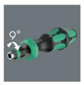
The bitholding screwdriver has a ratchet mechanism integrated in the handle - with its fine toothing it has a small return angle and thus allows fast working.
