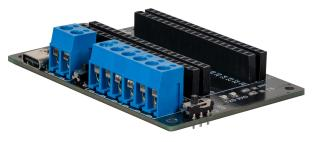
This expansion board allows you to add an RS485 and a CAN interface to a Raspberry Pi Pico.
