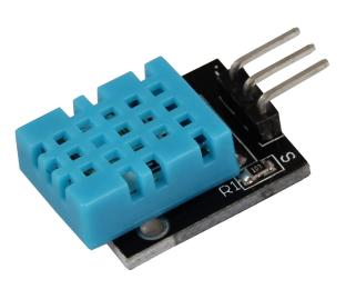
This sensor is a combination of temperature sensor and humidity sensor, united in one compact design. Here, however, the sampling rate of the measurement must be taken into account, since only every two second a new measurement result is available to you. Therefore this sensor is particularly suitable for long-term measurements.
