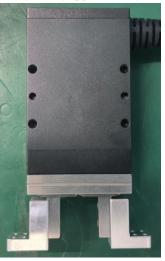
2. Install the gripper fingers and tighten the screws. Adjust the installation position of the gripper fingers on the L-shaped adapter according to the actual situation. The protective pad on the side of the gripper fingers can be attached or removed as needed.
