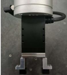
3. Connect the gripper cable to the end-of-arm aviation connector.
