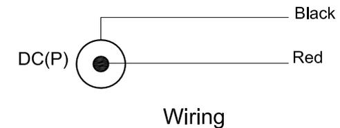
Voltage/Current Max.:12VDC 3A
