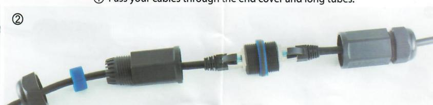
② Connect your patch cords to the RJ45 coupler in central tuber, assemble the long tubes on the central tuber, lock the two waterproof plugs on the cable, then put them into the end of the long tube. Screw the end covers (sealing cap) at both ends onto the long tubes.
