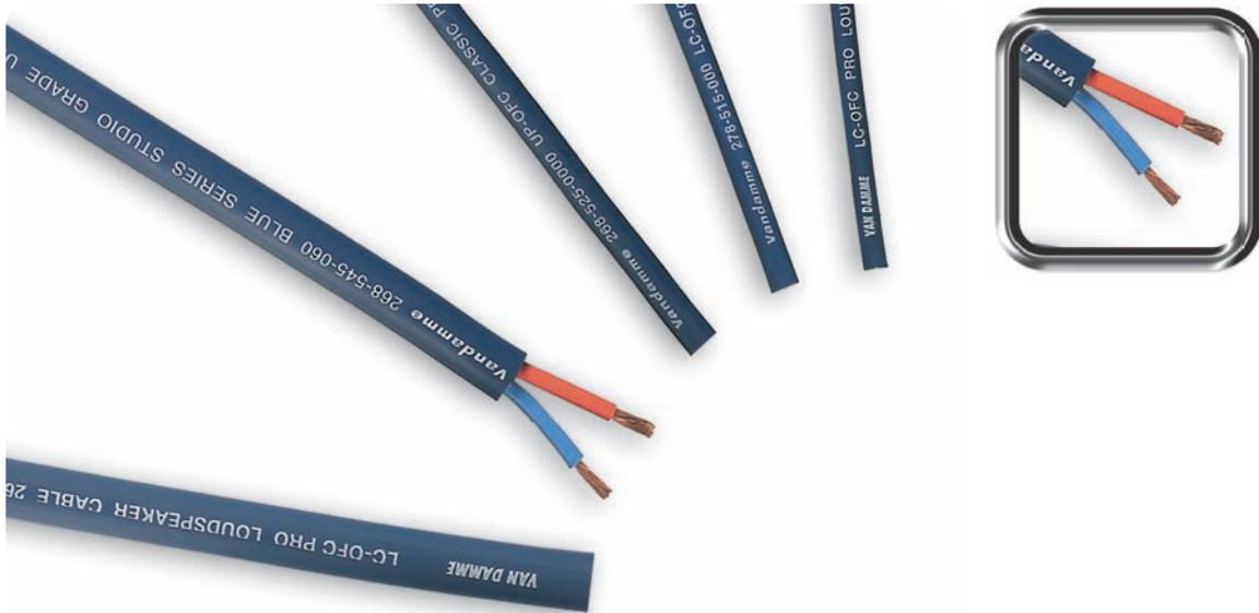
Van Damme Blue Series Studio Grade Speaker Cable caters not only for the recording studio environment but also for the rehearsal studio, live and presentation markets. All are twin-axial types and range from 0.75mm conductors for 100V line through to 6.00mm conductors for long runs of low impedance speaker signals.
