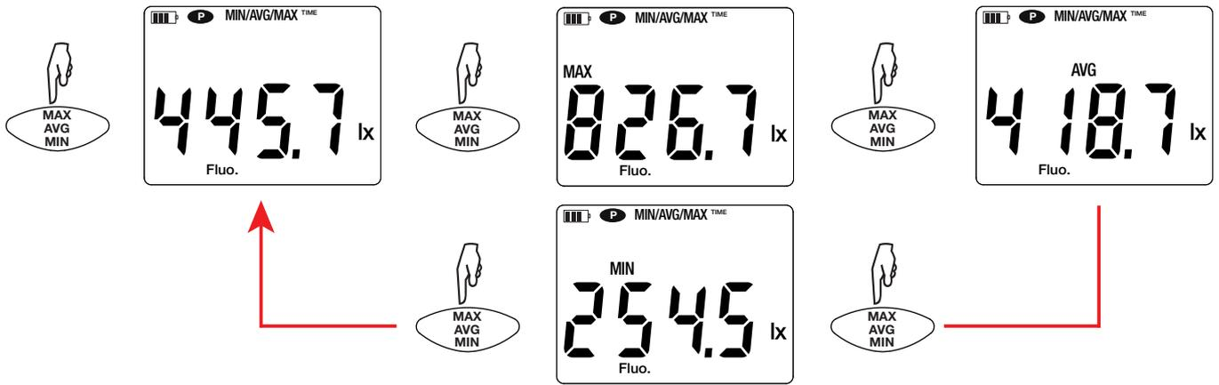
To exit from the MAX AVG MIN mode, long-press the **MAX AVG MIN** key.
