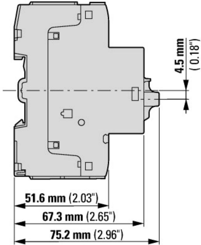
Motor-protective circuit-breaker with standard auxiliary contact
