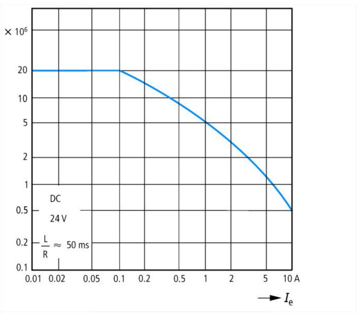
$$\label{eq:component lifespan (operations)} \begin{split} & l_e = \text{rated operational current} \\ & \text{Three contacts in series} \end{split}$$
