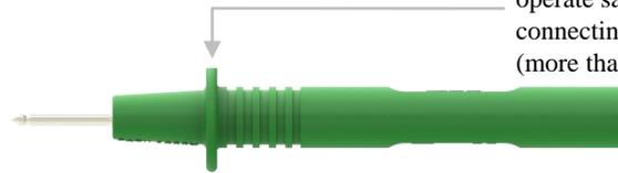
Barrier. Keep behind this barrier to operate safely the product while connecting to hazardous live voltages (more than 30 V AC and 60 V DC).
