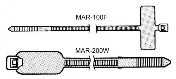
Partex Marker Ties provide a quick and effective method of securing and marking bundles of cables. They can also be used for component marking and pipe identification. Markings can be made using any indelible marker. Available only in natural (clear) colour.
