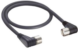
M23 Power Double-Ended Cordset: Male angled to female angled, 19-pin, black body, 120 V AC/DC, 16x8 A + 3x10 A; PUR black cable, 16x0.5 mm<sup>2</sup> + 3x1.0 mm<sup>2</sup>
