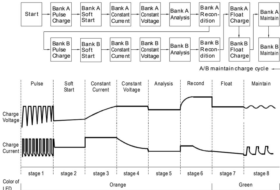
Figure 6.3 8 stage charging curve
