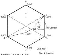
Sample: G5Q-14 12 VDC Number of Relays: 5 pcs Test conditions: Shock is applied in ±X, ±Y, and ±Z directions three times each with and without energizing the
