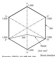
Sample: G5QU-1A-HR-HA-VH Number of Relays: 5 pcs Test conditions: Shock is applied in ±X, ±Y, and ±Z directions three times each with set and reset status to check the number of contact malfunctions.
