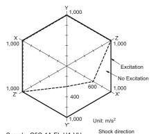
Sample: G5Q-1A-EL-HA-VH Number of Relays: 5 pcs Test conditions: Shock is applied in ±X, ±Y, and ±Z directions three times each
