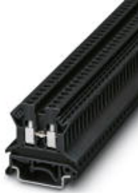
Feed-through terminal block, Connection method: Screw connection, Cross section: 0.2 mm 2 - 4 mm 2 , AWG: 24 - 14, Width: 5.2 mm, Color: black, Mounting type: NS 35/7,5, NS 35/15
