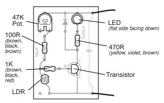
To make the LED light up when the sensor is in bright light the positions of the LDR and the potentiometer should be swapped. A different value potentiometer may be needed, depending on the sensitivity required.
