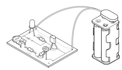
This general purpose light sensing circuit uses a mini light dependent resistor (LDR) to detect changes in the level of light. It is designed for use with a 3V - 9V battery. When the components are connected as shown below, the LED will light up when the sensor is in darkness. The sensitivity of the circuit can be set by adjusting the potentiometer.
