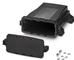
Empty enclosure for wall or mast mounting, black (9005), modular electronics housing with front plate, for outdoor applications, degree of protection: IP66/IP67/IP69, width: 164 mm, height: 180 mm, depth: 64 mm, PCB surface: 13160 mm<sup>2</sup>
