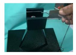
4. Fix the gas pipe in the air hose provide under the launcher, Just push fit.
