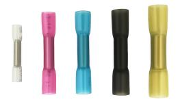
**Technical data:** Shrink ratio: 3 : 1 • IP-Class: IP 67 • Temp.-range: -55 °C ... 125 °C • Voltage resistance: max. 600 V • Shrink temperature: 80 °C ... 130 °C • Glue melts during shrink-process.
