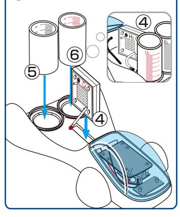
Remove the cap from each tube connected to the fuel cell. Using the syringe, inject distilled water into the Oxygen side of the fuel cell until the fuel cell is HALF filled with water. WARNING: The polymer membrane is an important part of the proton exchange membrane (PEM) fuel cell, it should be prevented from drying out.
