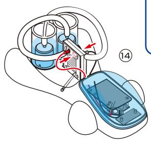
Connect the red and black cables to the solar panel, and connect the other ends to the red and black sockets on the fuel cell.
