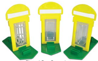
Clip and Cage Frame devices standing in base locators
