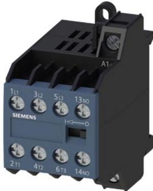
Powerrelais, AC-3 8,4A, 4kW / 400V 4S, AC 230V, 45...450Hz 3 polig, Schraubanschluss
