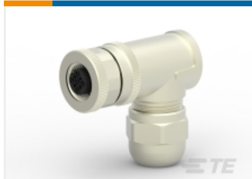
TE Part #T4112011041-000 M12 F, 4P GOLD A_CODE RA SHIELDED PG7
