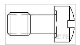
D-Shaped Connector Accessories: Mounting Screw
