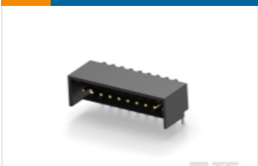
TE Part #2-644488-2 Polyester Right Angle PCB Header: 2.54mm, Shrouded, With Mating Alignment
