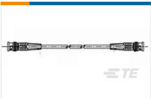
TE Part #1337771-4 50 OHM COAX BNC STR PLUG STR P
