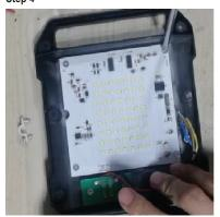
Unscrew 4x light source board screws.
