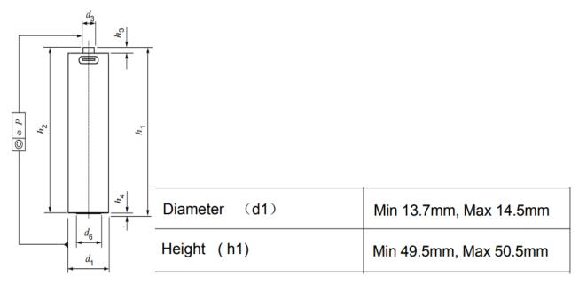
Capacity: 1300 mAh (130 mA, 25°C, e.v.= 1.1 V)
