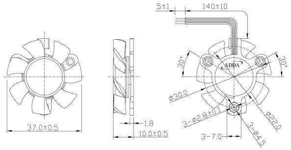
LEAD WIRES : UL 1571, AWG30, L =  $140 \pm 10$  mm Red = positive ; Black = negative.
