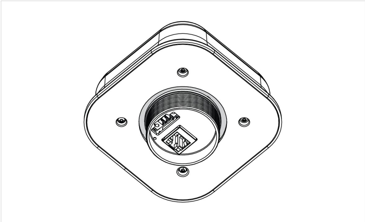
3. In the mounting surface, drill a mounting hole with the size  $\varnothing$  M50 (50,5 mm).
