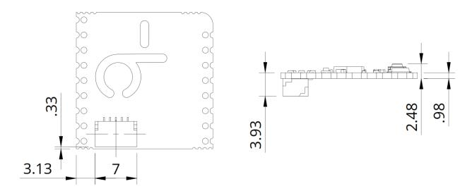
The Nicla Sense Env was designed to be usable as a surface-mount module and presents a dual inline package (DIP) format with the MKR-styled header connectors on a 2.54 mm pitch grid with 1 mm holes.
