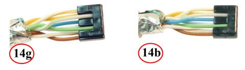
Slide load bar to end of pairs to make loading into housing easier
