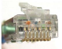
Verify wires are visible through end of plug
