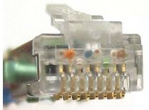
Verify wires are visible through end of plug
