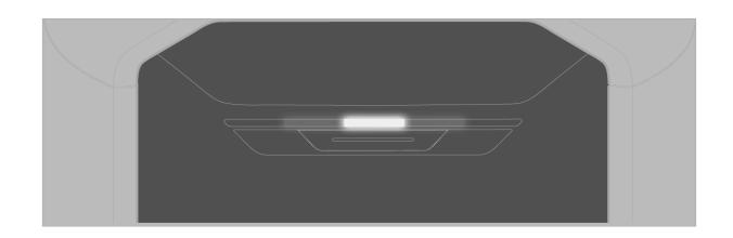
When the status LED light is solid, the number of LEDs that are lit up indicate the current battery level.
