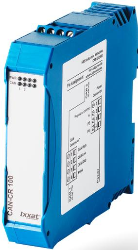
The CAN repeater CAN-CR100 with integrated bus termination resistors and two CAN/CAN FD interfaces can be used to improve the load capacity of the CAN bus with nodes, physical coupling of CAN/CAN FD bus systems or to insert a galvanic isolation.
