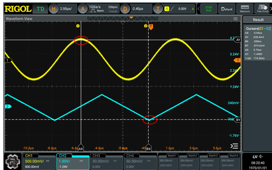
Figure 10.13 Track Measurement (after Horizontal Expansion)
