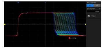
Segmented memory collection will store the waveform into multiple memory segments (up to 80,000) and each segment will store a triggered waveform as well the dead time information. The interval between segments can be as small as 2  $\mu$ s. All segments can be played back using the History function.
