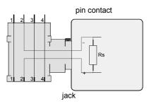
If the 'signal/GND'-line in your transmitter is not assigned to contact 2, please do not forget to adjust the logger-angle-type plug and the external angle-type plug accordingly:
